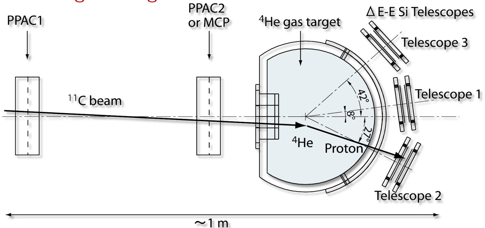
Measurement:  Beam position   $E_{beam}$   Proton position   $E_{proton}$
