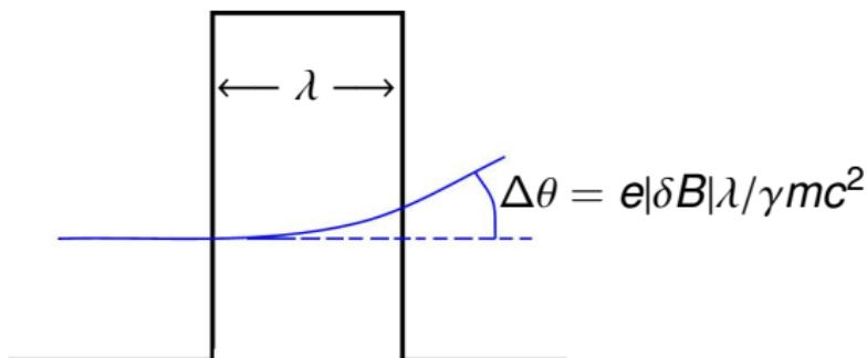
Define strength parameter  $a \equiv \frac{e|\delta B|\lambda}{mc^2}$ : ratio of deflection angle to beaming angle
