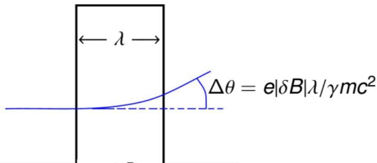
Define strength parameter  $a \equiv \frac{e|\delta B|\lambda}{mc^2}$ : ratio of deflection angle to beaming angle
