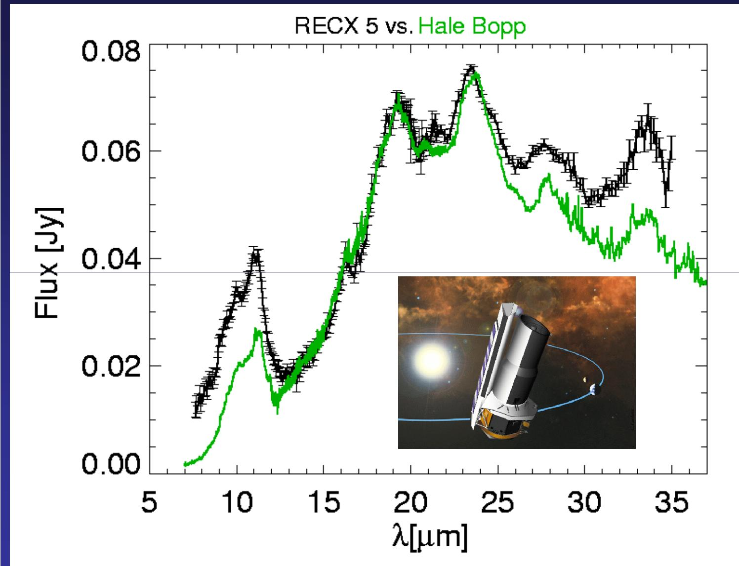
IRS (5-40  $\mu\text{m}$  long slit, R=150, 10-38  $\mu\text{m}$  echelle, R=600)
