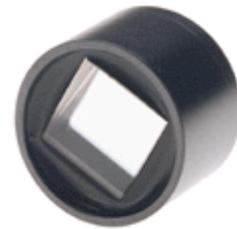
These prisms are used in medium power applications requiring high transmission and a high degree of polarization purity. Like the Glan Laser prisms they are air-spaced to minimize absorption losses. The two prism sections are mounted in absorbing black glass within the cell.
